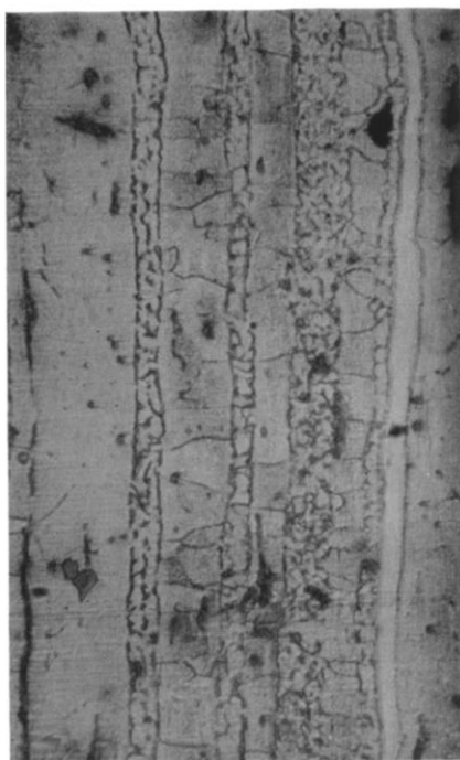
Figure 2. Microphotographs of the Cross-section of an Indonesian Kris. (2a) Transverse, (2b) Longitudinal. (Original 20X)
